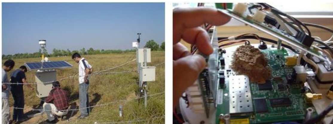
Figure 1. Field Server installed on 2007 December 24 (left) and Insect nest built on CPU board of Field Server(right).
