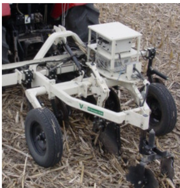
Figure 1. (left) Veris shank-based spectrophotometer for near-surface mapping.
