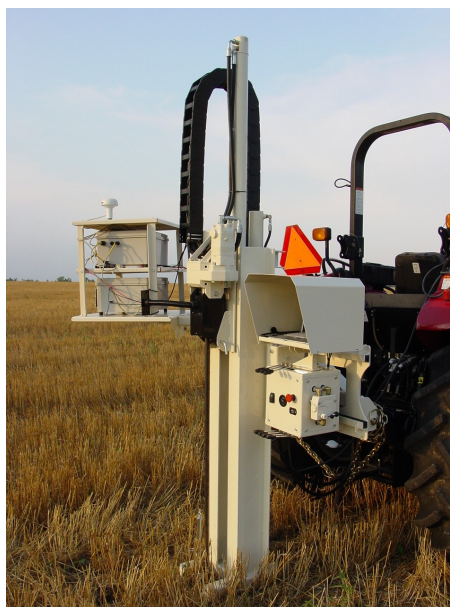
Figure 2. (right) Veris probe-based spectrophotometer for profile measurements.
